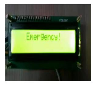
The LCD display can exhibit the text message when controlled by an Arduino-equipped smart glove is shown in the above fig.
