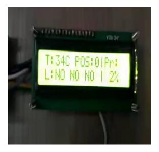
By utilizing a combination of temperature sensor, pressure sensor, and accelerometer with an Arduino UNO, the body's position, air pressure, and temperature can be accurately identified is shown in the above fig.
